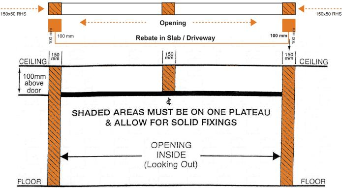
Note: orange sections must be solid fixing - no gaps and must be load bearing.
