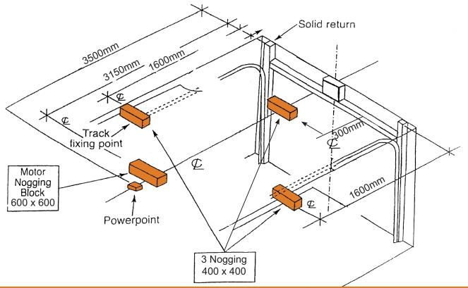
**Note:** Roof noggings must be packed down flush with plaster ceiling - **no gaps.**Floor rebate must be 100mm back from finish opening and 100mm in width from opening.
