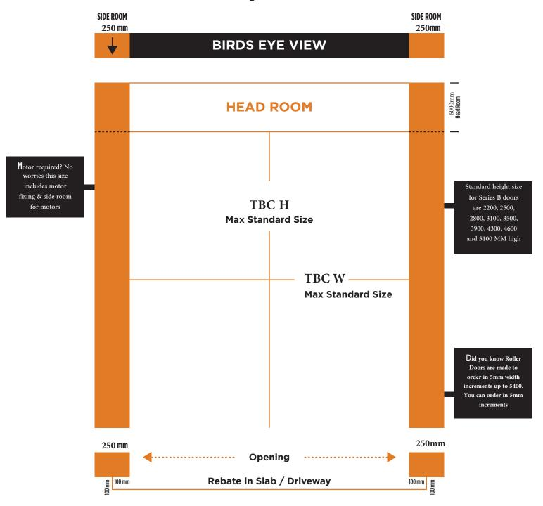
Solid fixing in orange no gaps. Fixing area to be one flat surface. For the best seal on the ground we need a 100 X 100 mm rebate in the concrete. BAL required? We can supply an Emb-A-Seal so your door is compliant.
