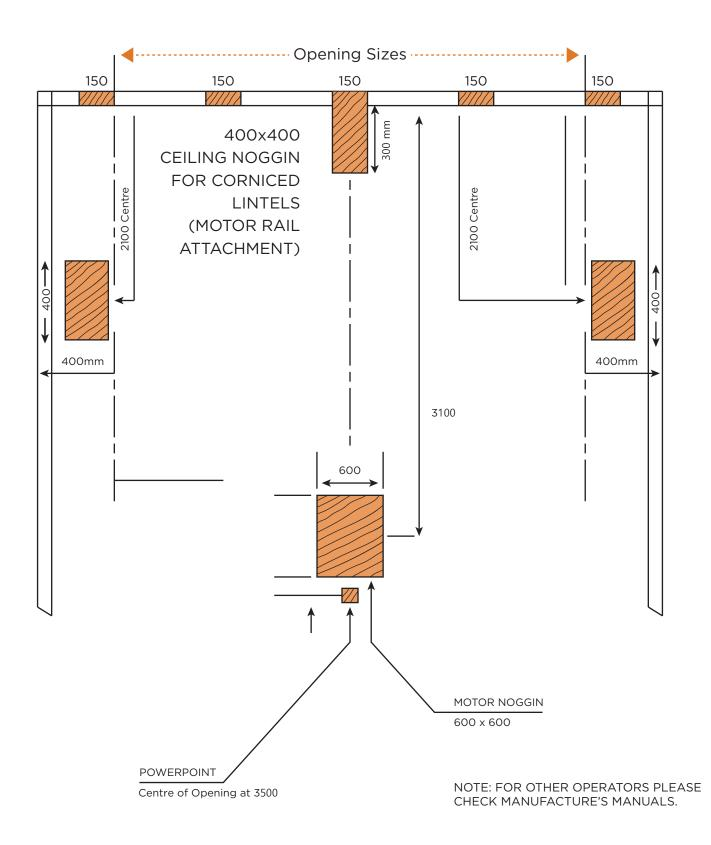
**Note:** Roof noggings must be packed down flush with plaster ceiling - **no gaps.** Floor rebate must be 100mm back from finish opening and 100mm in width from opening. Opening must be one flat surface. Save this sheet to our IBook's now for future reference.
