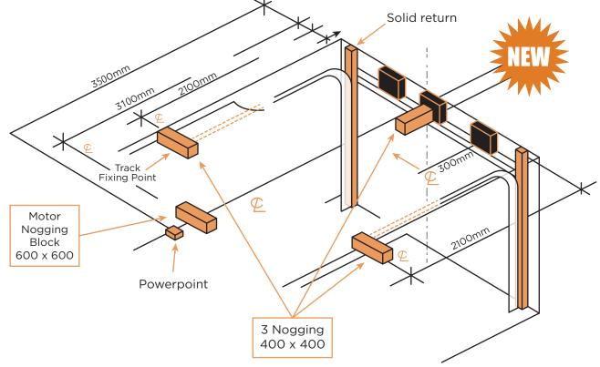
**Note:** Roof noggings must be packed down flush with plaster ceiling - **no gaps.** Floor rebate must be 100mm back from finish opening and 100mm in width from opening. Opening must be one flat surface. Save this sheet to our IBook's now for future reference.
