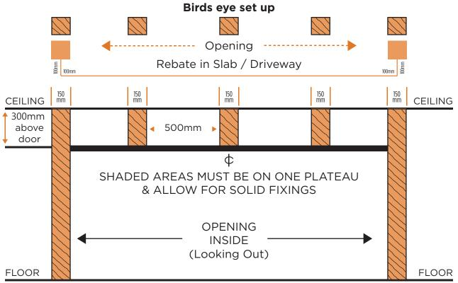
Note: orange sections must be solid fixing - no gaps and must be load bearing.
